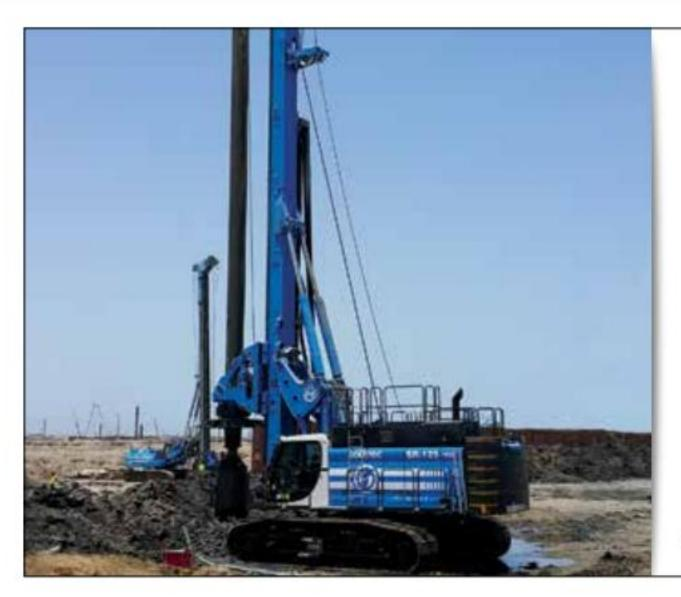
The new **SR-125 HIT** is designed for bored piles, CFA, CSP (double-head cased auger piles), displacement piles, soil mixing and Turbojet<sup>®</sup>.
